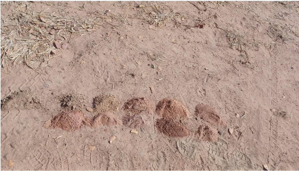
soil samples taken at every 5 meters of drilling.
